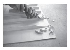
From our series of Ruckers construction pictures: Shaping the ends of the ribs
